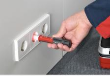
Test wall sockets for AC voltage and polarity
