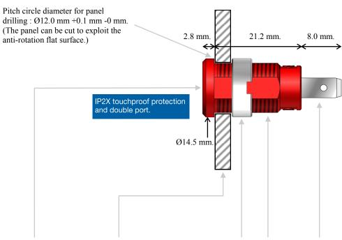
The 4 mm banana female connection complies with the panel 4 mm banana plugs of most of the worldwide most famous manufacturers and meets the requirements of interchangeability dimensions of the French standard NF C 93-440:1986.
