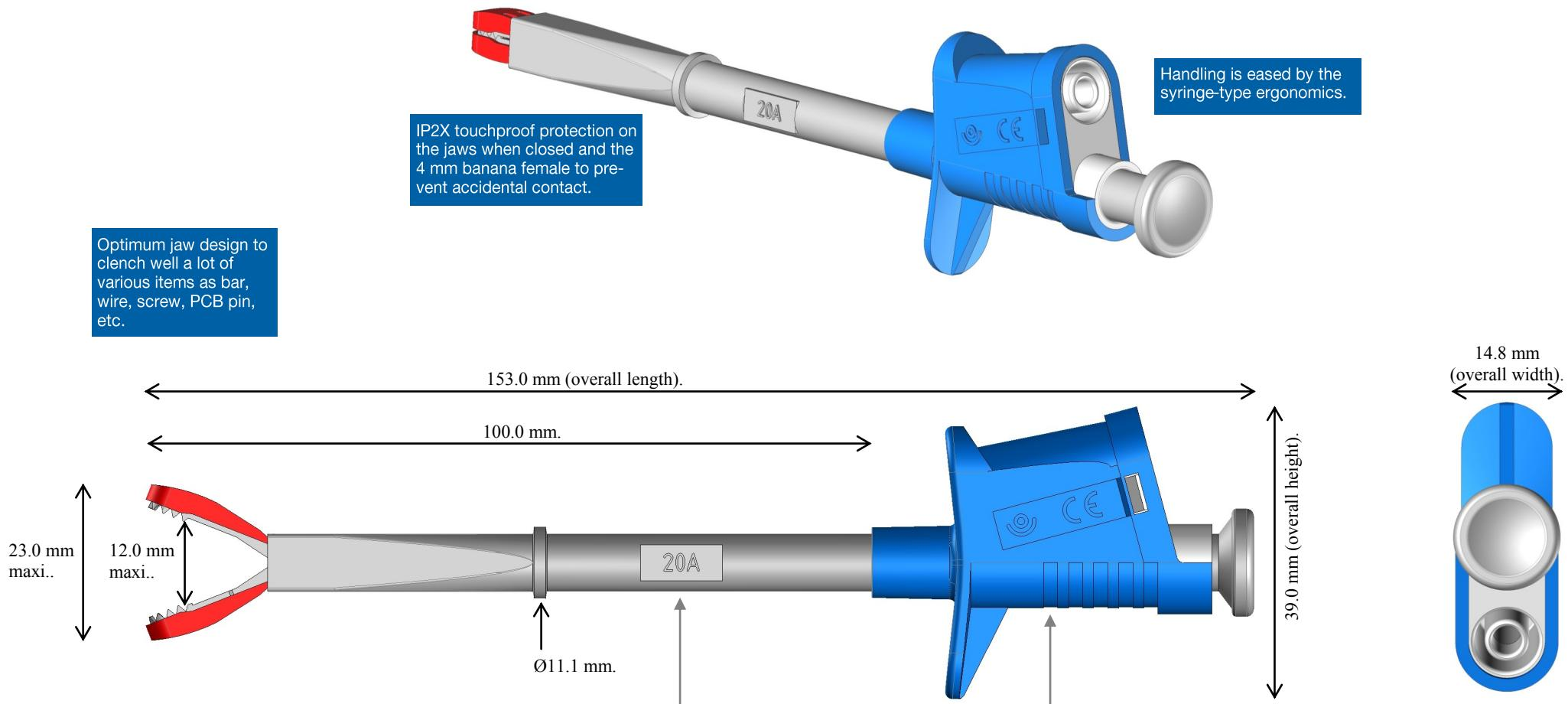
With the flat end of the stem and the shape of the clip various target items can be clenched and the electrical contact is reliable.
