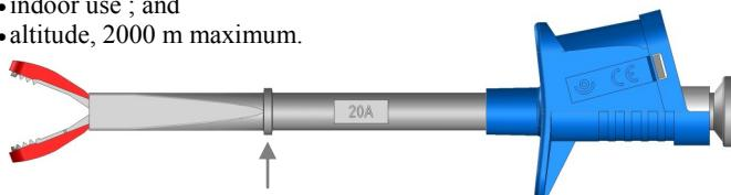
Barrier. Keep behind this barrier to operate safely the product while connecting to hazardous live voltages (more than 33 V AC and 70 V DC).
