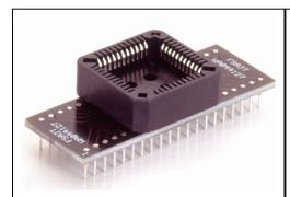
This is a complete range of Adapters which coverts a PLCC package to either an PGA or DIL footprint.
